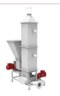
Dedicated to sticky/pasty products or filter cakes, this dryer is fitted with two counter-rotating rotors at its bottom where hot gases are injected through a Venturi nozzle.
