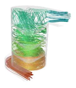
Cyclonic dryer is composed of a cylindrical body with a set of internal conical baffles. Wet product is introduced into the air stream through a Venturi feeder. Gas-solid mixture is tangentially fed at the bottom of the dryer.
