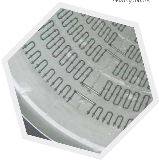
▼ Detail of electrical heating mantel
